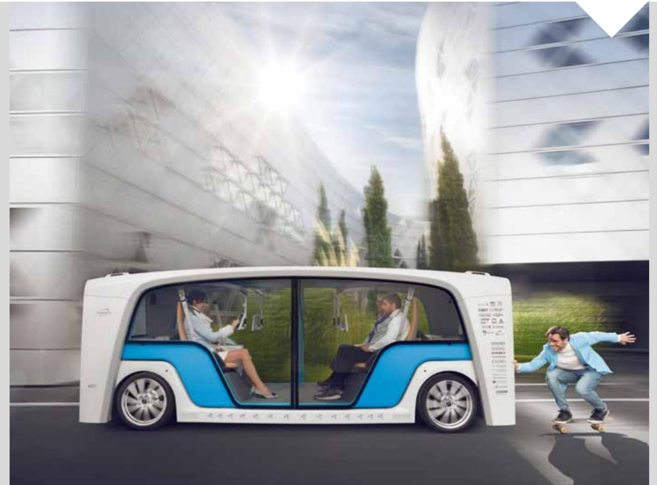
"snap". In this way, the different lifecycles of mechanical components and components susceptible to wear and aging such as IT hardware can be separated from the "car or transport cabin" and can be connected temporarily through a simple "click" for passenger transport or other transport services. "Skateboard" and "pod" would, however, be only temporary companions – always depending on the mode of transport. What would be the advantages of this innovative relationship for the automotive industry?
